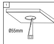
**Step 1 -** Cut a hole in the ceiling with a diameter of 55mm.
