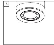
**Step 5 -** When properly installed, the recessed spotlight will clamp against the ceiling/ frame.
