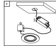
**Step 4 -** Connect the spots in series via the distribution box. Connect the loops to the empty connectors.
