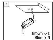
**Step 3 -** Connect the phase and zero wire, to the L and N side of driver.(indicated on the driver/trafo).
